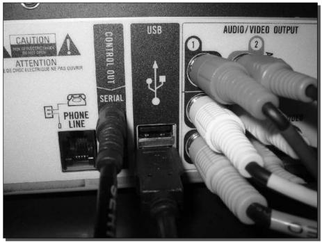
FIGURE 12-4: TiVo Series 2 sports two USB ports. Either should work fine.
