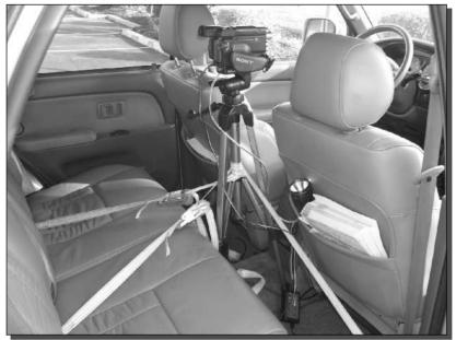
FIGURE 14-17: Camcorder tripod strapped to the passenger seat.
