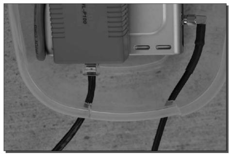
FIGURE 8-18: Cables exit the case without strain or pinching.
