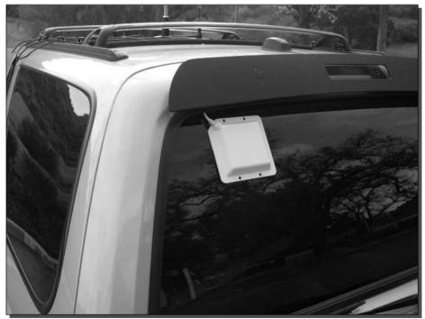
FIGURE 14-15: Directional panel antennas mounted on the cars.
