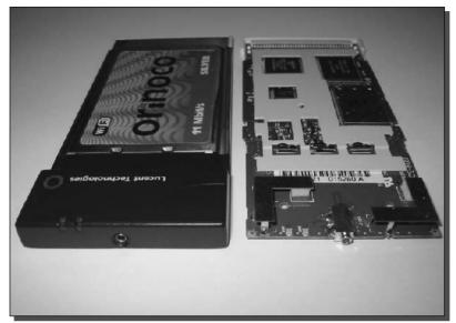
FIGURE 5-3: External connector and internal antennas on the Orinoco PC card.
