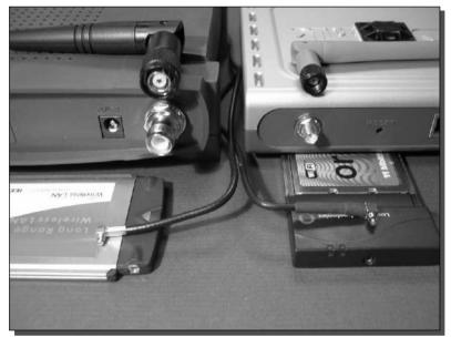
FIGURE 1-27: Various Wi-Fi connector types.
