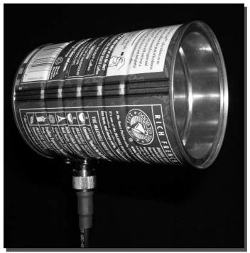
FIGURE 3-2: The tin can waveguide antenna.
