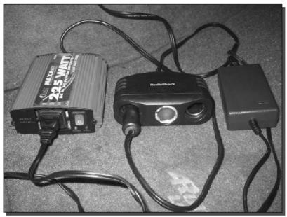
FIGURE 5-12: DC adapter, DC-to-AC inverter, three-way splitter. This rig can run forever.
