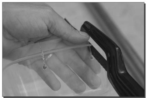
FIGURE 8-17: Drill the case first, then cut down to the holes.
