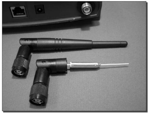
FIGURE 2-5: A cut-away interior of a popular coaxial antenna.
