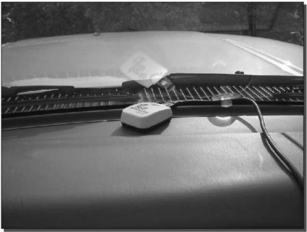
FIGURE 5-15: The dashboard makes a nice home for this USB GPS.
