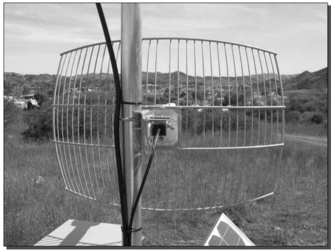
FIGURE 13-5: A parabolic dish antenna.
