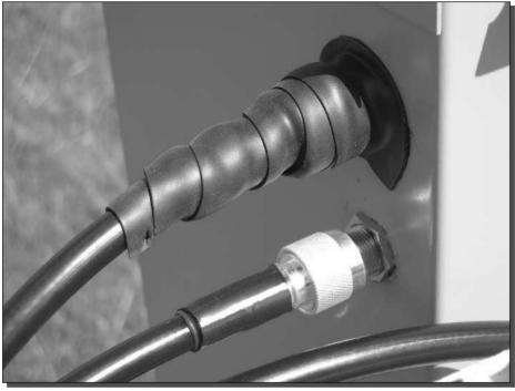
FIGURE 9-23: Sealant tape protecting microwave connectors.
