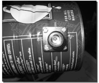
FIGURE 3-17: The connector mounted in the can.
