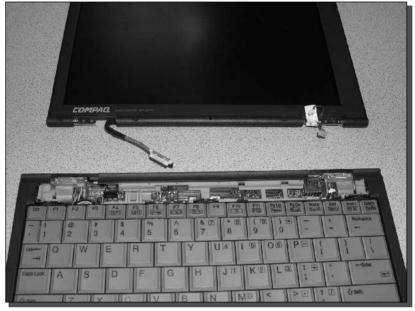
FIGURE 15-10: LCD panel removed.
