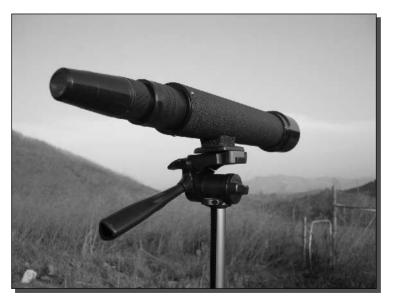
FIGURE 13-4: Spotting scope used to determine direction and angle.
