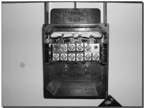
FIGURE 9-6: The junction box built in to the Shell SP75 solar module.
