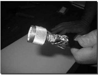
FIGURE 1-22: Connector and pin are in position.
