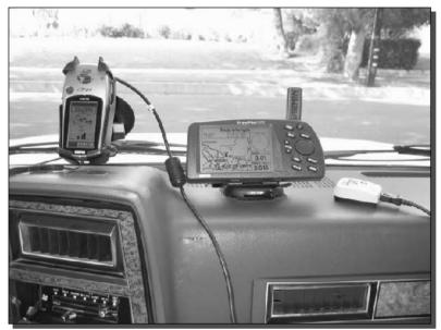
FIGURE 5-7: Handheld, dash-mounted, and dedicated GPS receivers.
