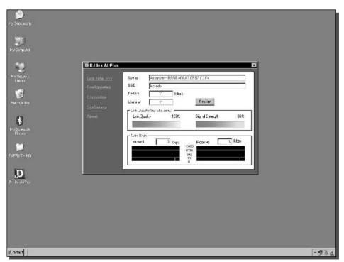
FIGURE 2-23: Signal strength survey in progress.
