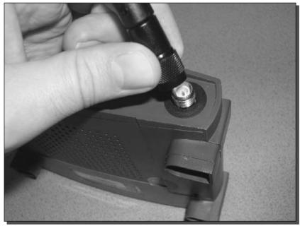
FIGURE 4-12: Removing the original antenna.
