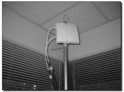
FIGURE 4-18: Antenna on a pole during a site survey test point.
