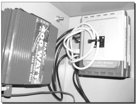
FIGURE 9-15: Wireless radios in place and connected via an Ethernet crossover cable.
