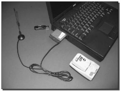
FIGURE 5-2: Equipment setup for a typical war drive.
