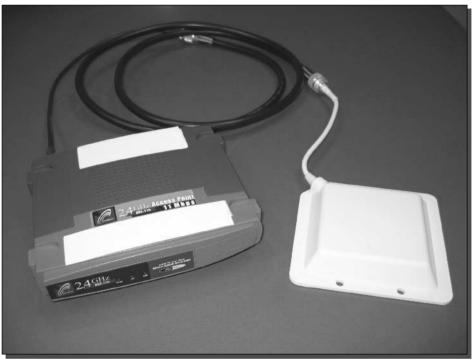
FIGURE 4-1: System using a Linksys WAP11 with a high-gain external antenna.
