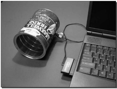
FIGURE 3-19: The completed can antenna hooked up to a laptop.
