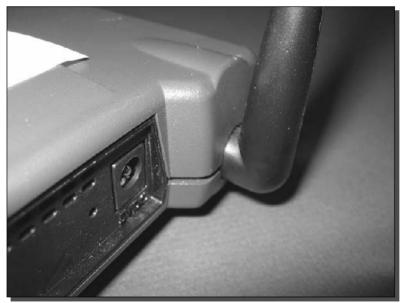
FIGURE 4-13: Cisco access point with a soldered antenna connector.
