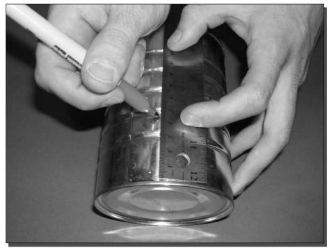
FIGURE 3-6: Marking the correct location for the N-Connector.
