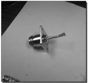
FIGURE 3-15: A bashed-out round connector with a wedge end.
