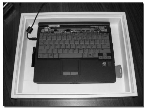
FIGURE 15-4: Laptop mounted in the frame with a PCMCIA Wi-Fi card.
