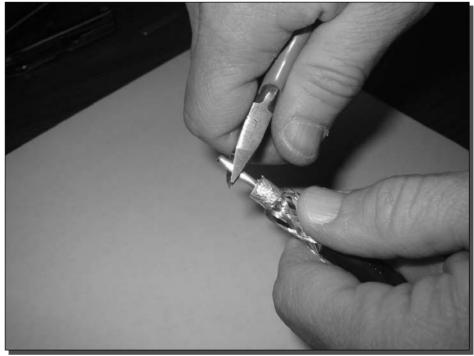
FIGURE 1-18: Clipping the core conductor.
