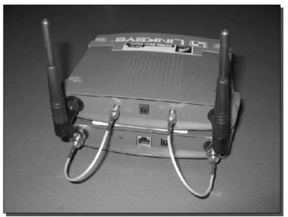
FIGURE 4-19: Linksys WSB24 adds power to a Linksys access point.
