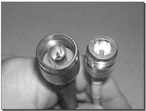
FIGURE 4-14: Standard male connector (left) and standard female connector (right).
