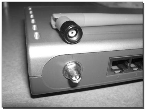
FIGURE 4-16: Reverse Polarity SMA connectors.
