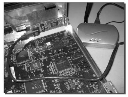
FIGURE 12-2: Series 1 TiVo with installed TurboNet adapter and Ethernet-to-wireless bridge.
