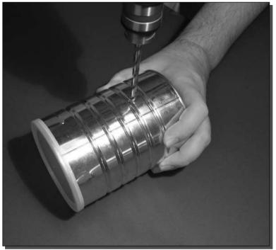
FIGURE 3-7: Drilling a hole in the can.
