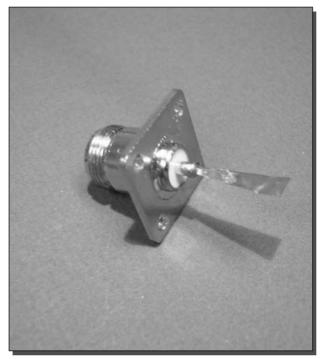
FIGURE 3-16: The completed Connector/Element assembly.
