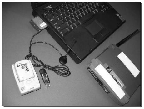
FIGURE 11-1: AP games hardware: laptop computer, wireless client adapter, wireless access point, and GPS receiver.
