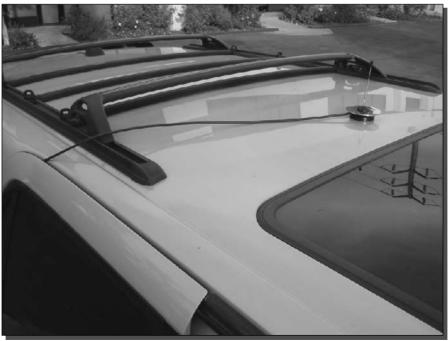
FIGURE 5-14: Magnet mount antenna placement with cable running through doorway.
